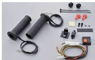
87478 4-level Heat Control For \Phi 22.2\text{mm} ( 7/8" ) motorcycles Open end
