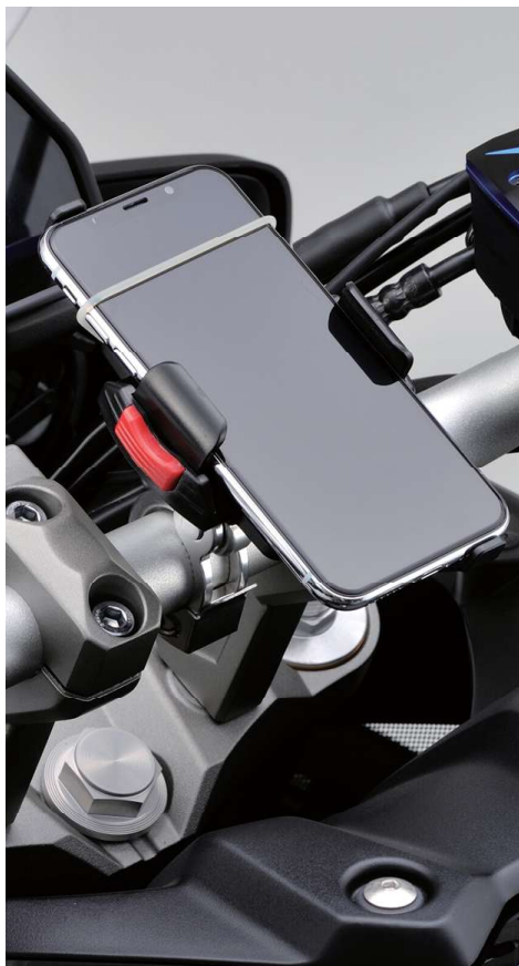
#87963 RIGID TYPE (bolt-mount clamp) #87964 DETACHABLE (quick-release clamp)
